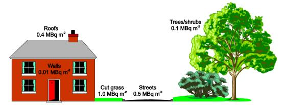
Figure 7.1 Contamination levels of <sup>137</sup>Cs on the various types of surface in the city for the hypothetical scenario given in Example 1
